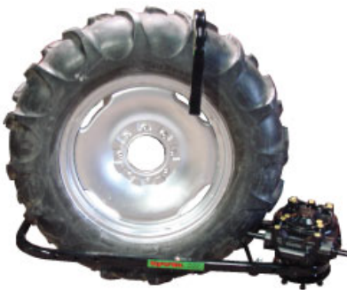
GEARBOX AND PIVOT TIRE SECURED FOR HAULING
